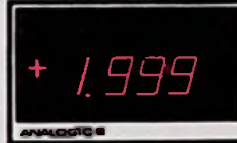
stroom DC 4-20 mA of 10-50 mA
